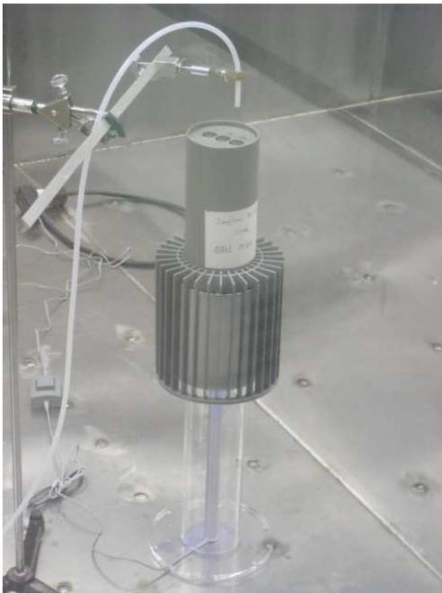
ON w/ charged particle collector installed
