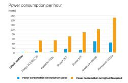
At full power, lonFlow air purifiers use only 5 watts compared to 60-175 watts for typical filter-based air purifiers. Since the air stays clean only as long as you do something about it, air purifiers should operate 24/7.
